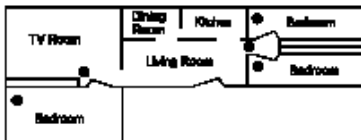
Figure 2: IN FAMILY LIVING UNITS WITH MORE THAN ONE SLEEPING AREA, A SMOKE ALARM SHOULD BE PROVIDED TO PROTECT EACH SLEEPING AREA IN ADDITION TO ALARMS REQUIRED IN BEDROOMS.
