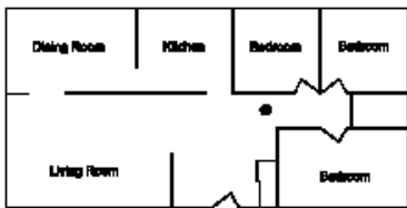
Figure 1: A SMOKE ALARM SHOULD BE LOCATED BETWEEN THE SLEEPING AREA AND THE REST OF THE FAMILY LIVING UNIT.
