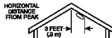
Figure 5: RECOMMENDED SMOKE ALARM LOCATION IN ROOMS WITH SLOPED, GABLED, OR PEAKED CEILINGS.
